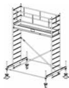
Working height: 4.40 m Scaffold height: 3.40 m Platform height: 2.40 m
